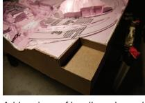
26. Build a spot for your power pack train control on one corner by cutting the hardboard and using the pieces to frame the area.
