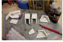
34. Sand or carve the edges of the plaster culverts and assemble each using super-type glue. A super glue "accelerator" ("Zip
