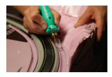
21. Once your track is in its final position (but not yet glued down), use a knife or hot foam cutter to carve drainage ditches on both sides.
