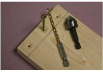
2. Use a drill to make pilot holes for the drywall screws. Follow up with a countersink to make sure the screws lie flat
