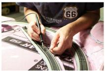
29. Use a 25-watt soldering pencil and 60-40 rosin-core solder to solder the rail joiners of each section of track together. This
