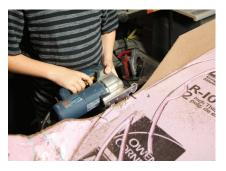
24. Use a jig saw to cut the hardboard even with the contours of the foam insulation board scenery.
