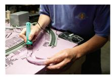
16. Carve out the top piece of foam insulation for the river bed. Use a knife, hobby knife, or hot foam cutter (shown here).
