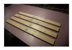
1. Cut two of the 8-foot 1x4s in half, to produce four 4-foot long pieces. These will become the frame for the layout.
