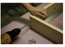
3. Create the layout frame by gluing, then screwing the four 1x4s together using drywall screws. Be sure each corner is square.
