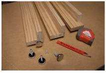
7. Cut four of the 1x4 and 1x3 boards to 48" in length and glue them into an "L" shape. These will be the legs. Drill the bottom of
