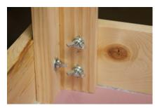
9. Drill through the frame and legs and attach them using three bolts, adding washers and wingnuts on back.
